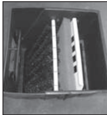
Fig. 35 SK900PRO with one row of brushes and the mat in middle position. (Net not shown)
