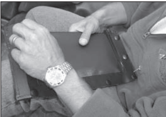
Fig. 19 Insert the ratchet fasteners into bellows from the outside of flap.
