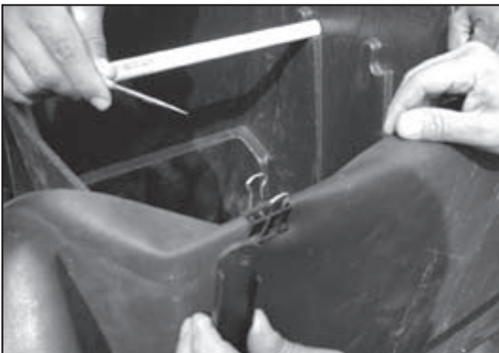
Fig. 13 Install the “U” frame using an awl to help align the holes.
