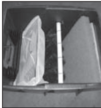
Fig. 34 SK700PRO with one row of brushes and the mat in rear position. Use with external pumps.
