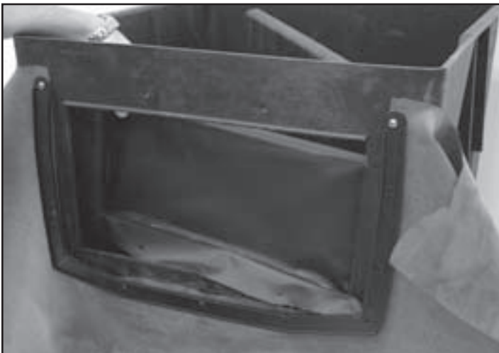
Fig. 26 Pass the bellows flange through the opening from the inside, placing it on top of the liner and between the liner and the frame.
