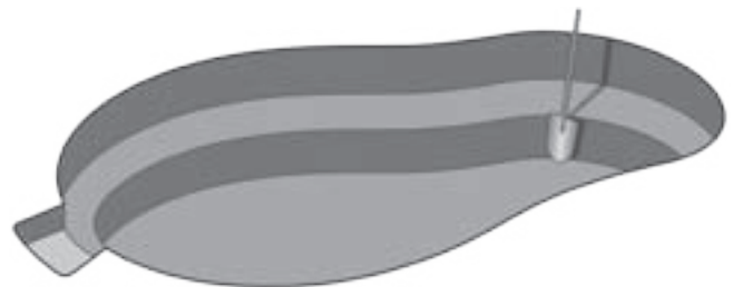
Fig. 4 Dig second shelf one shovel depth and start excavation of skimmer hole.
