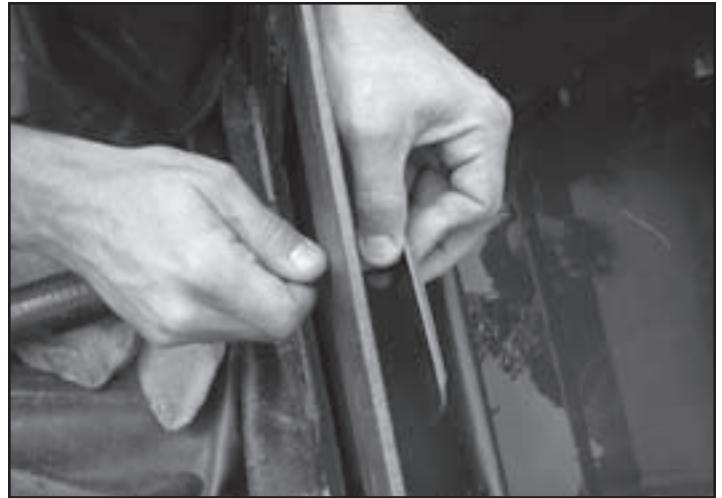
Fig. 22 Install the latch tab with the supplied nut and bolt.
