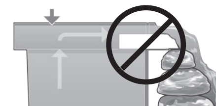
Fig. 22 If a thick rock along with a larger flow pump is used, the water flow may be so great that it will flow over the sides of the Endless Cascade™ vault.
