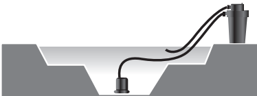
A. Above ground, pumped back into pond.
