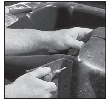
Fig. 6 Using an awl, poke a hole through the liner at the screw holes.
